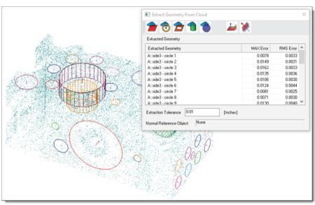
A second surface circle extraction option has also been added that allows a user to detect geometry within a specifed proximity to a set of nominals and build the fit geometry from point clouds where only the surface can be scanned (such as is the case when working with sheet metal). This function does not require CAD, but can use a set of reference geometry directly as guidance.
