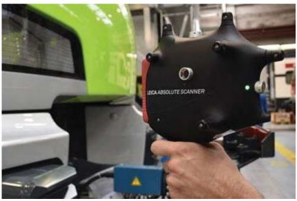
The new portable LAS-XL is a new ultra large-scale portable laser scanner and runs in the tracker interface, like the LAS. The LAS-XL requires RDS v.4.3.
